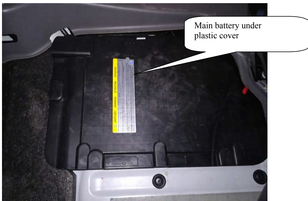
Fig. 6. Location of main battery
