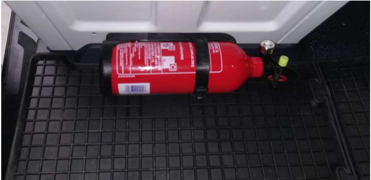
Fig. 47 Driver's compartment fire extinguisher
