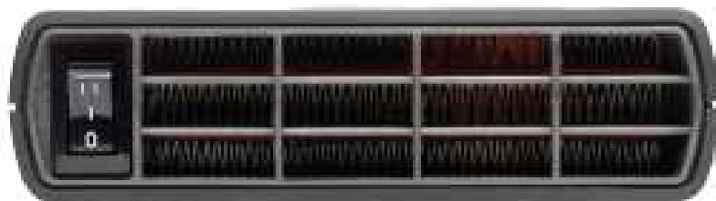
Fig. 26. DEFA 2100 thermoelectric heater with three-position power switch The interior heater is attached to a bracket from which it can be easily removed by pulling in the direction of the air outlet, and reattached by sliding the heater onto the rails of the bracket in the opposite direction to that of removal.
