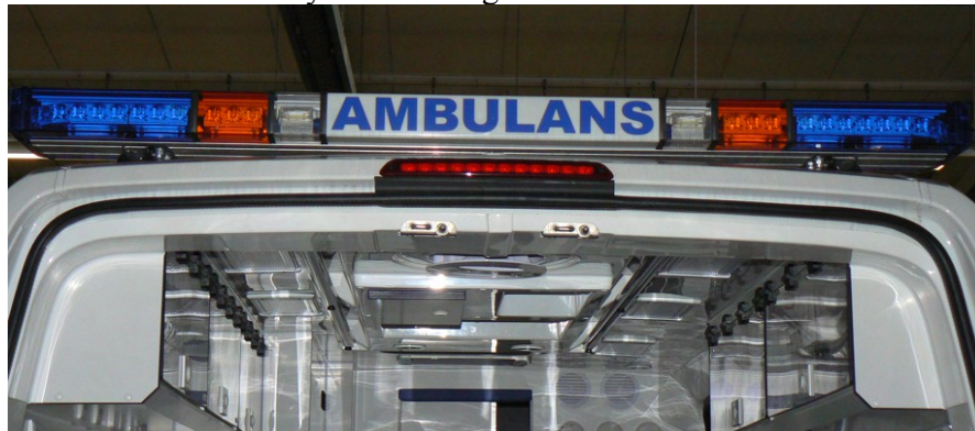
Fig. 30. Work lights integrated with priority lighting - rear of ambulance
