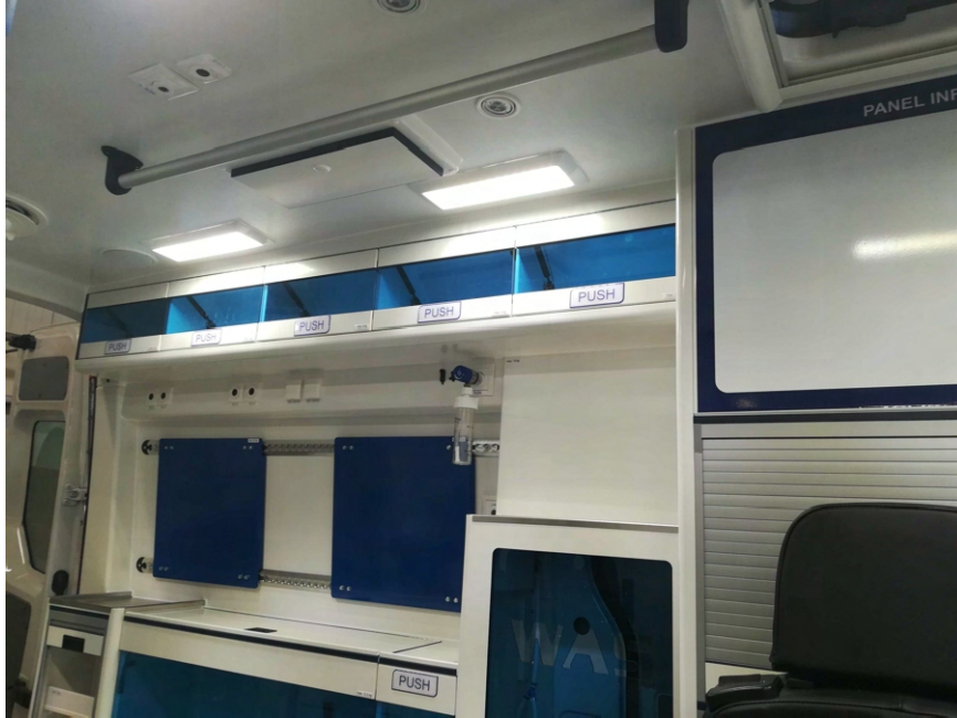
Fig. 35 Oxygen sockets with oxygen humidifier
