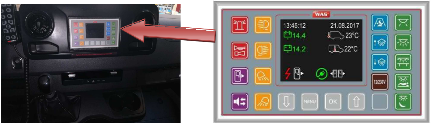
Fig. 17. Location of the control panel in the driver's cab
