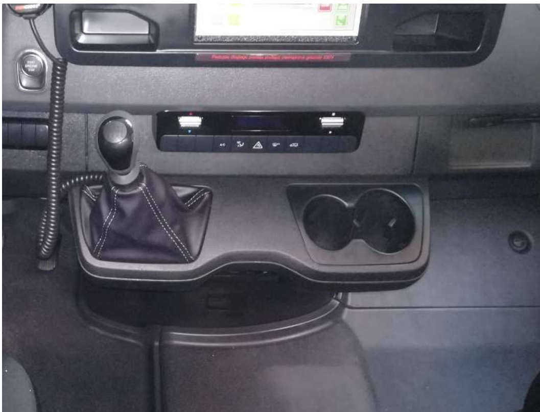
Fig. 21 Location of the button for activating the driver's compartment air conditioner
