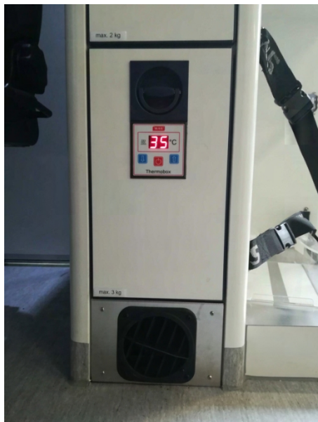
Figure 28: Storage compartment with IV fluid heating function "Therobox".
