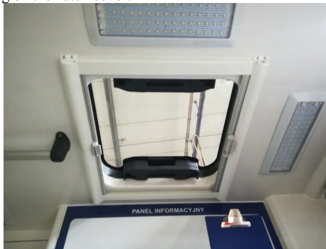
Fig. 54 Manual roof hatch installed in the medical compartment
