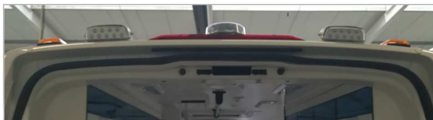
Fig. 31. Additional work lights with direction indicators
