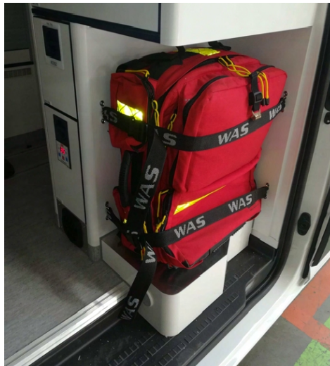
Fig. 58 Medical bag recess at right sliding door.
