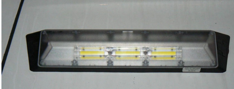
Fig. 29. Work lights located in housings integrated into the vehicle body - left and right sides of the ambulance
