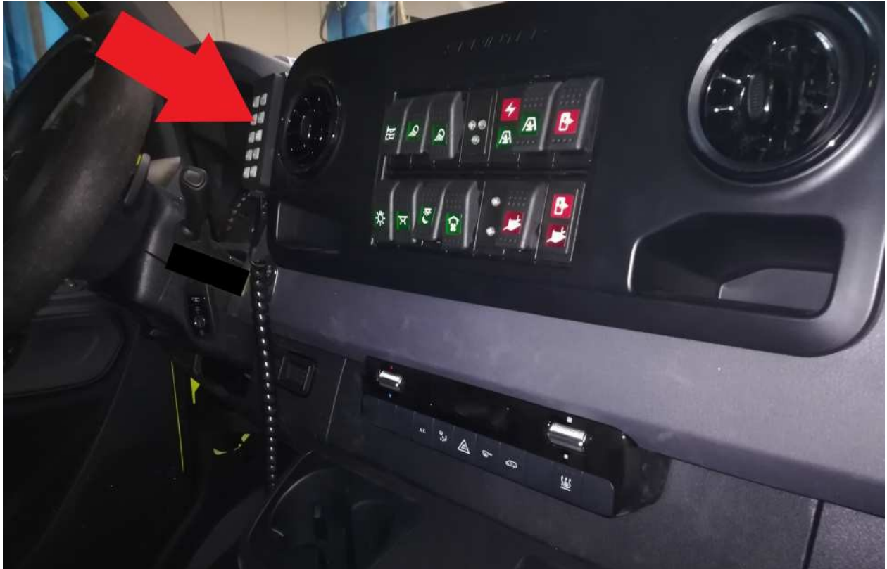
Fig. 32. Position of the manipulator in the driver's compartment
