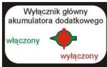
Fig. 14. Position label for secondary battery switch
