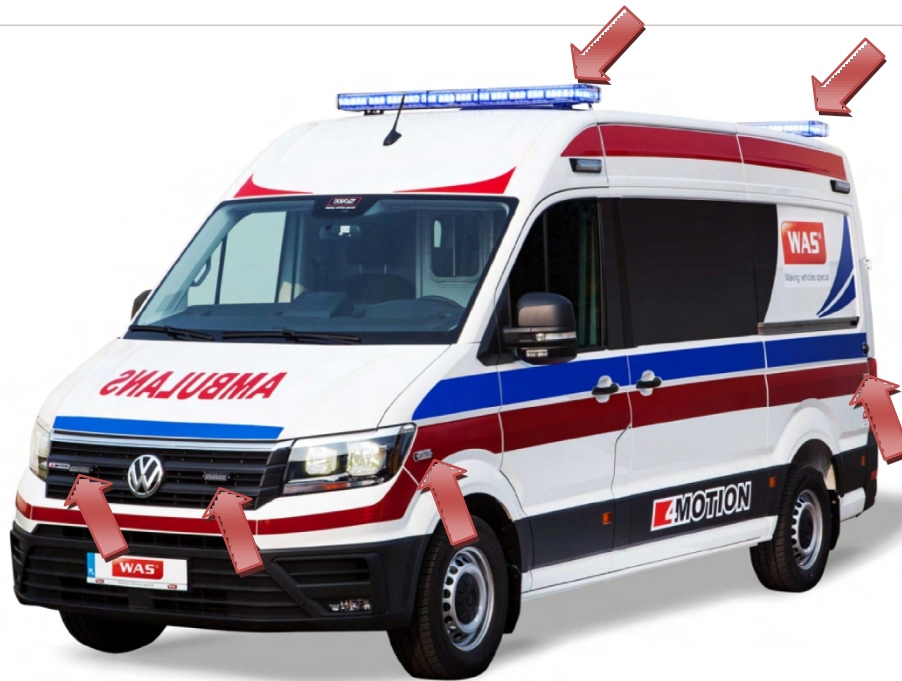
Figure 33: View of the ambulance with emergency lighting fitted.
