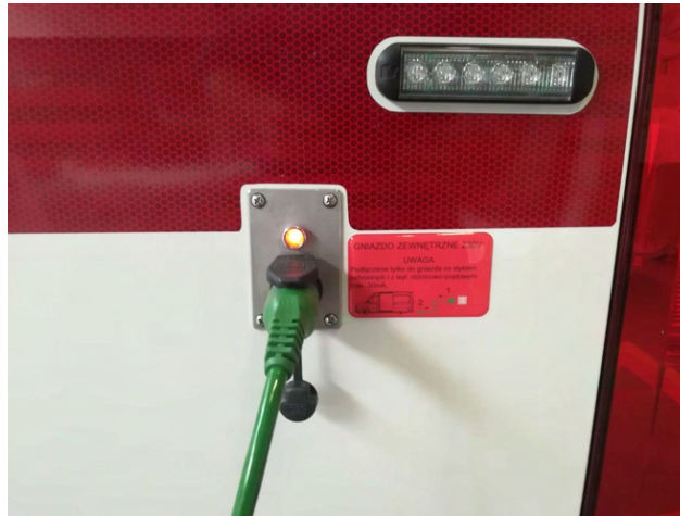
Fig. 66. Connection of external 230V power supply.
