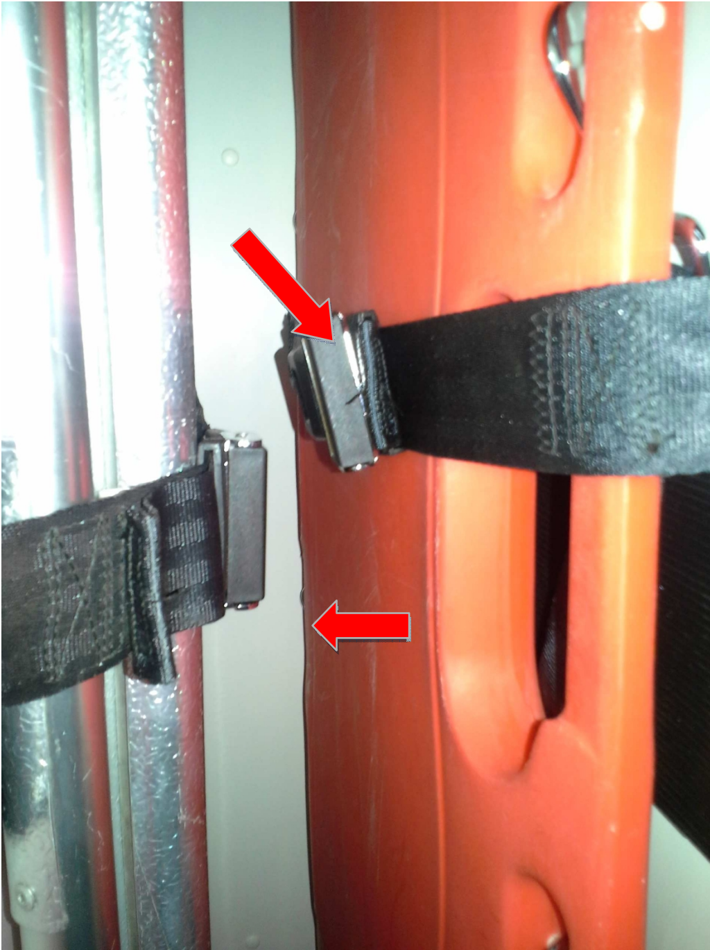
Fig. 65. Method of attaching the pick-up stretcher and orthopaedic board.
