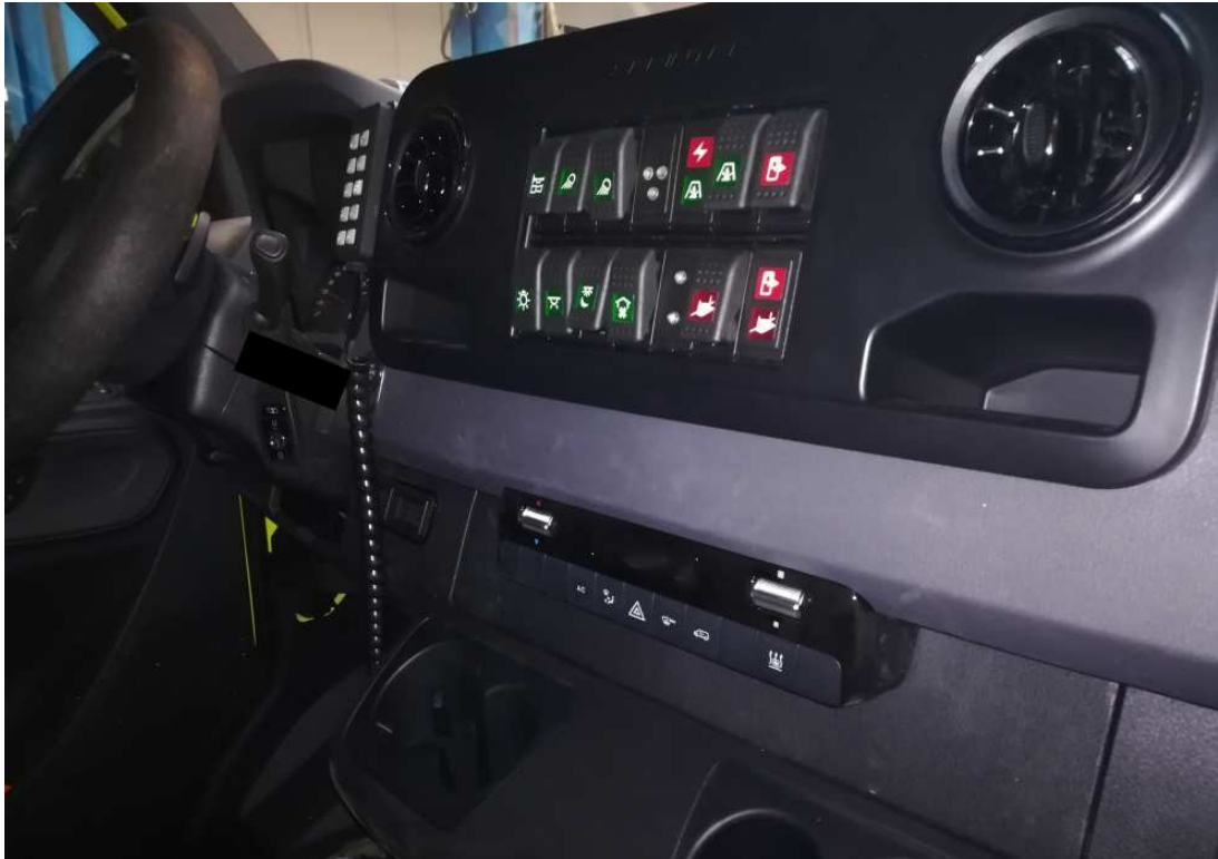
Fig. 18. Location of the set of controls in the driver's cab
