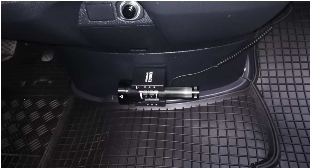
Fig. 41. Wireless searchlight in the driver's cab
