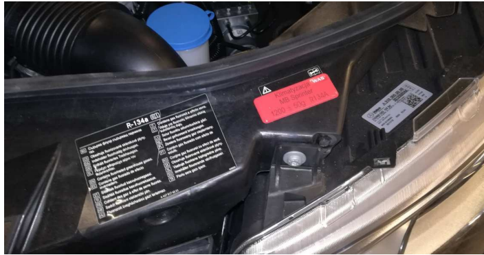
Fig. 23. Label in the engine compartment indicating the necessary amount of R134a gas.
