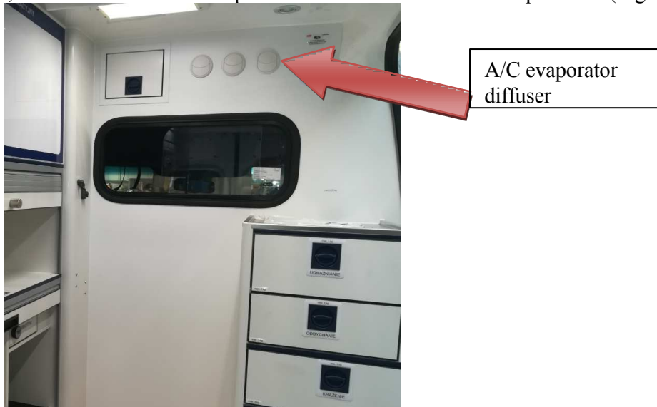
Fig. 22 Location of the medical compartment air conditioning evaporator with fresh air intake.
