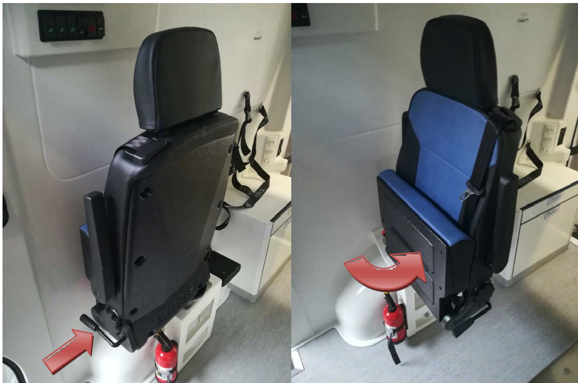
Fig. 50 Using the lever to rotate the seat through an angle of 90°
